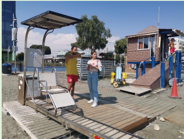
Image 1. Mr. Zenonos presenting us the Seatrac System designed by Tobeia, offering unassisted sea access to people with disabilities and mobility issues.
